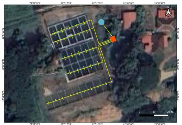
Schematic diagram location of ponds and tentative pipeline & water source point. (BLUE - circle: open well; RED rectangle - Pump shed, yellow lines : tentative pipeline across existing aquaculture ponds )
